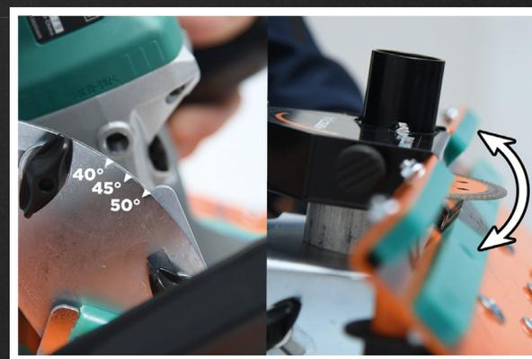
Adjustable cut for inclinations from 40° to 50°.
