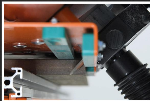
Adjustable bevel depth, with maximum cutting height of 21 mm, disc cover with dust extraction.
